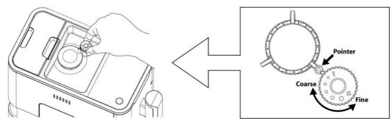
1. Only turn the knob for adjustment when the grinder is in operation.
