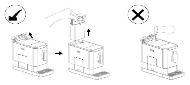
2. Rinse the water tank with fresh water and fill the tank to "MAX" level. Place it into the machine and make sure it is fully inserted.
